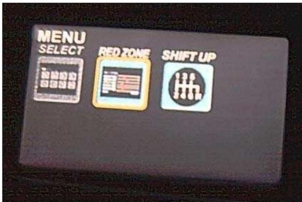
Pressing the **MENU** button when in mode 1 allows you to see the option screen again, with only the red zone and rev light options available. Use the **joystick** to navigate left or right to the **RED ZONE** option and **press the joystick** again to bring up the red zone screen. This lets you set warning points for each monitored sensor.
