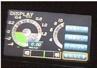
Display button, takes you into a menu to set brightness, auto-dimming, gauge peak tracking, and to turn the display off.
