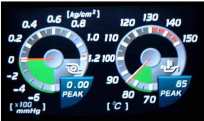
This mode lets you monitor any 2 gauges simultaneously (1 is permanently stored in RAM, the other 3 are use selectable). If you disconnect the battery or pull the fuse, you will find only the default pair available.
