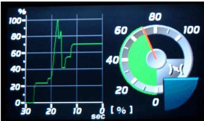
This mode lets you see 1 gauge and the last 30 secs of data from that sensor, with a peak hold function and peak value displayed in the blue segment (this does not apply to the throttle position sensor shown)
