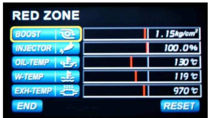
screen will switch back to Mode 1 from any other screen, and highlight which sensor went over the limit.
